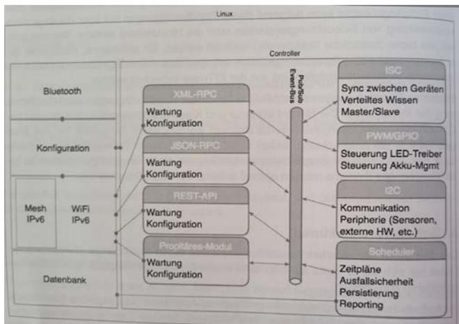
Fig.16: Example of software components of message-controlled intelligent lighting system; IOTware. [22]
