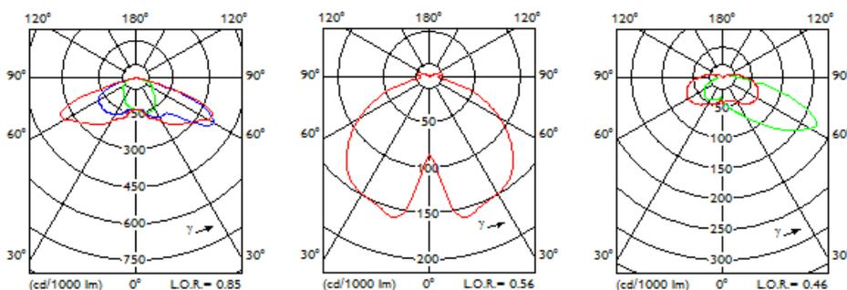
Fig.2: Typical light distributions in street lighting applications. [1]
