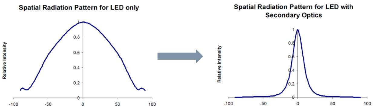
Fig.9: Change in light beam width using diverging optics. [4]
