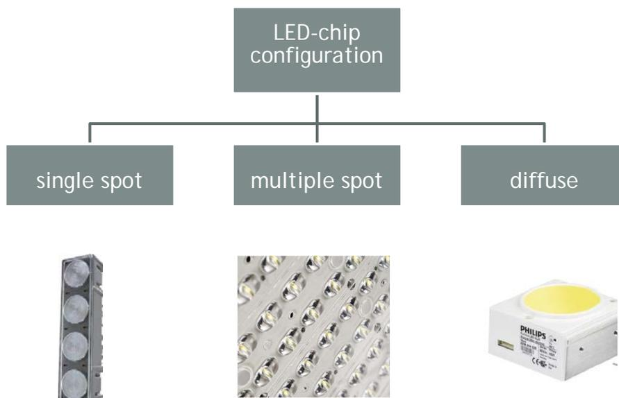
Fig.11: LED chip configurations. [1]
