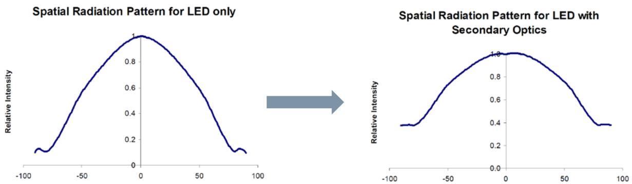
Fig.7: Change in light beam width using diverging optics. [4]
