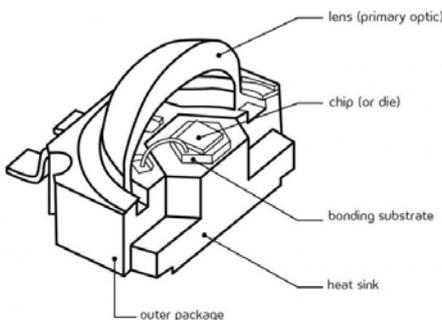
Fig.3: Typical LED package. [2]
