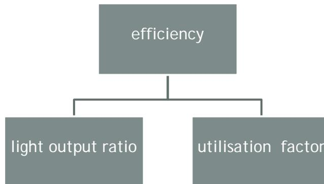
The Light output ratio (L.O.R) is a necessary property to define the efficiency of a luminaire. As the L.O.R approaches to one, more light will come out of the luminaire. This factor is the ratio between the luminous flux produced by the lamp to the luminous flux coming out of the luminaire. The differences between the two are termed as losses. Losses can be:
