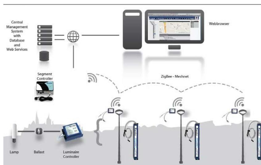
Figure 2: Principles of function of a wireless control system [28]
