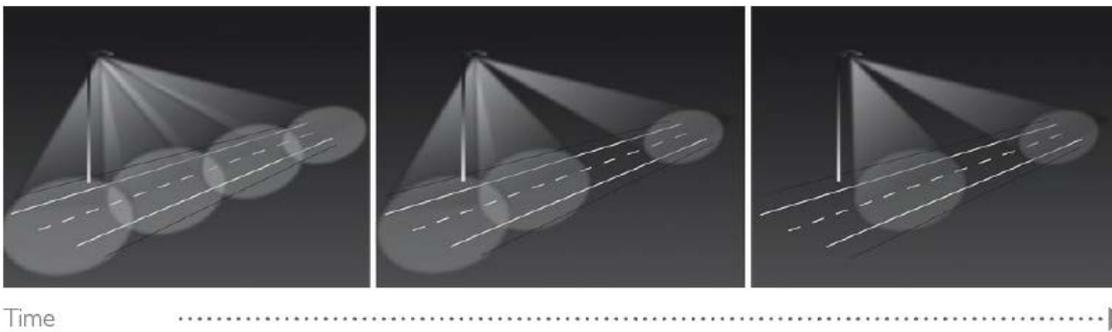
Fig.12: Dimming strategy: Multi-layer and Multi-spot. [1]
