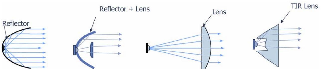
Fig.8: Collimator optics. [4]
