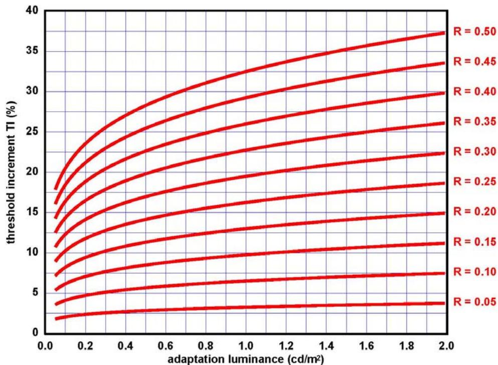
Figure 2: Threshold increment as function of adaptation luminance for different ratios  $R$  of veiling luminance to adaptation luminance
