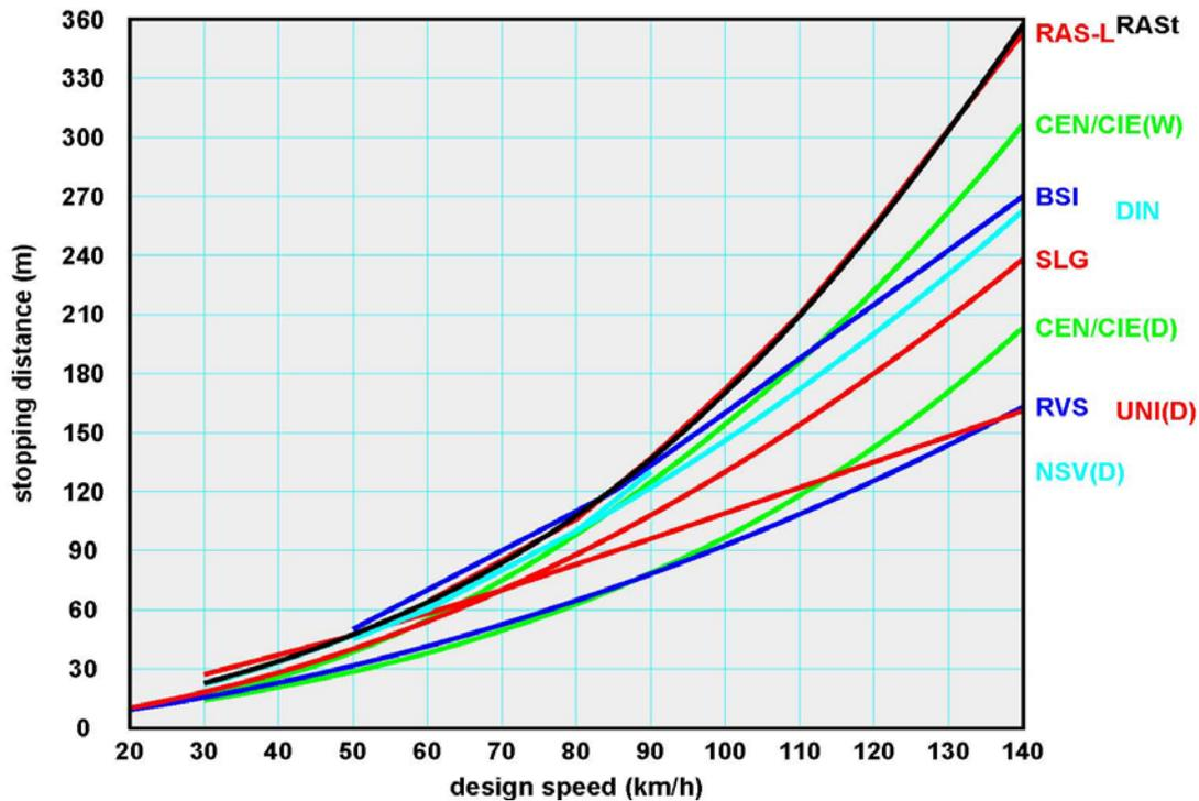
Figure 1: Stopping distance as function of design speed according to different national and international regulations [10]
