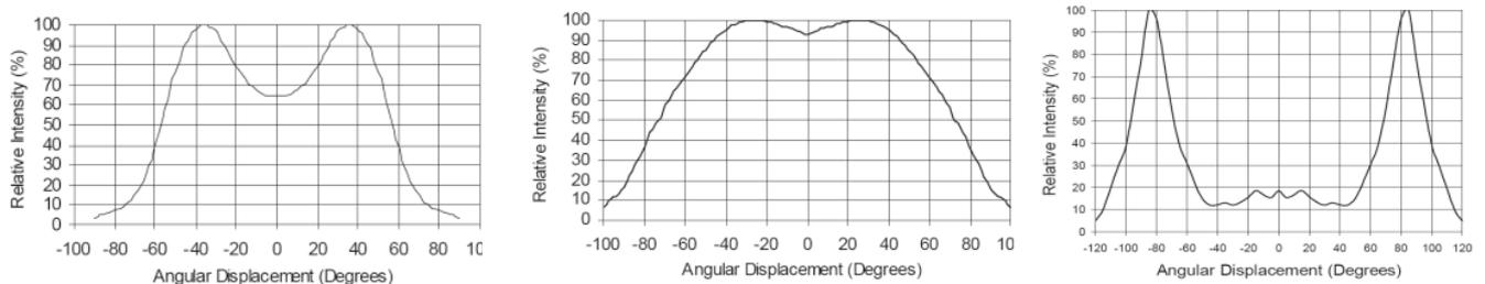
Fig.1: a. Batwing; b. Lambertian; c. Side-emitting. [1]
