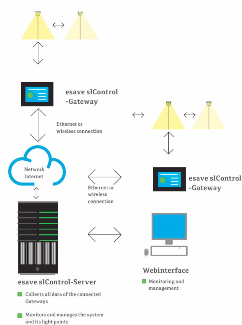
*Figure 7: esave sIControl – street light management solution*
