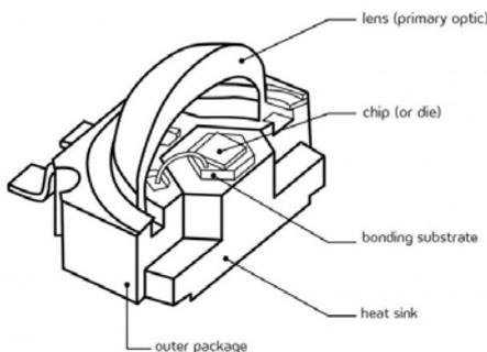
Fig.3: Typical LED package. [2]
