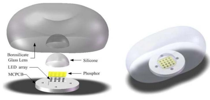
Fig.4: Primary optical system of LED chip array module. [3]
