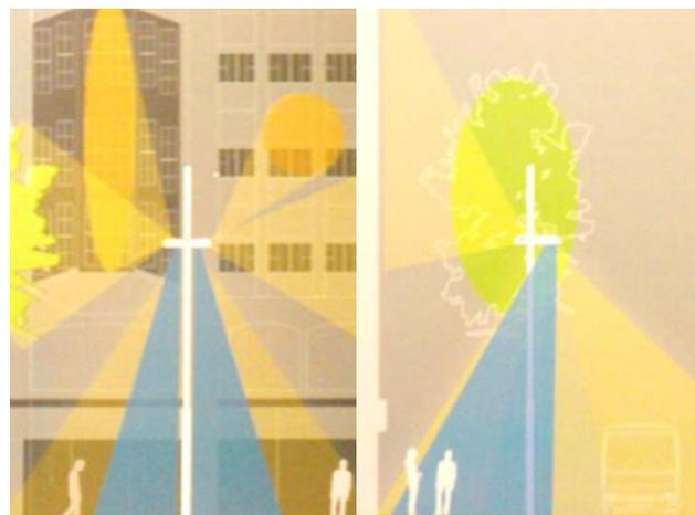
Fig.12: Multi-functional luminaires. [14]
