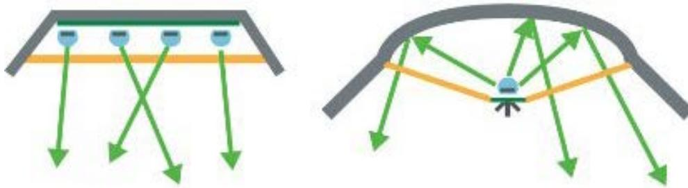
Fig.10: Change in light beam width using diverging optics. [4]
