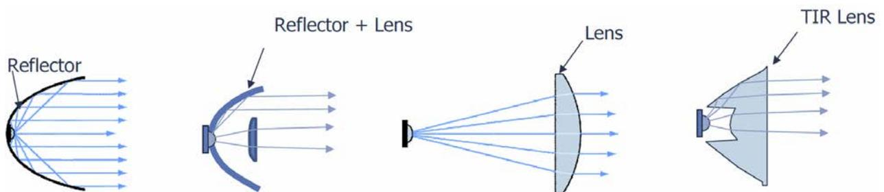
Fig.8: Collimator optics. [4]
